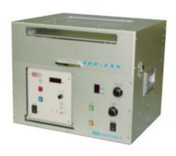
This test equipment enables evaluation of surface modification by corona treatment simply by setting a cut sheet of up to size A4 on the treatment table. Since the unit comes equipped with a ceramic electrode, it can test not only insulating sheets but also conductive sheets such as aluminum foil. An optional metal electrode kit (aluminum electrode and dielectric mat), exclusively for testing insulating base materials, is also available.
